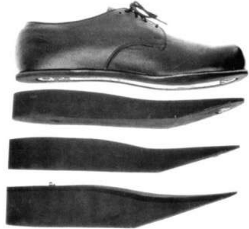
Fig. 2: The modular shoe used in the experiments. The upper and 3 different rocker bottom shoe modules are shown. For further details see Cavanagh et al. (1997) 1
